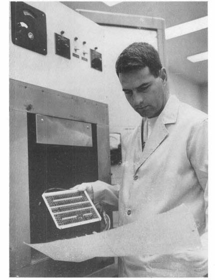
CHAMBER TEST — Ross R. French (7432-2) prepares a satellite logics system module for a temperature test. Small chamber provides heat-cold environment from  $-25^{\circ}$  to  $+175^{\circ}$  F. Module will also be connected with AGE tested for performance check while in the chamber.
